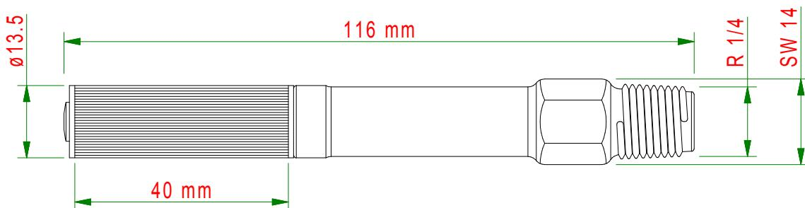
Injection packer with connecting thread R1/4" for 14 mm drill hole.
